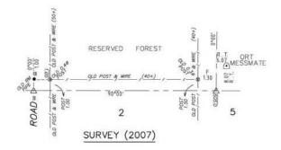
Survey by Forests Commission surveyors in 1950 defined the boundary between Reserved Forest and freehold Crown Allotment 2. Reference marks were placed at each end of the boundary as shown on the first diagram. The boundary was recently surveyed as shown in the second diagram.
