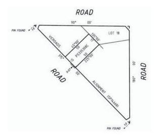
Say you were asked to re-establish Lot 18 on the same plan and registered survey PS335308C existed within the LP section. On inspection of PS335308C, you found that it was of limited extent, basically having re-established the Vicroads survey and maintained the LP dimensions.
