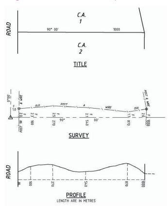
Survey of the boundary between Crown allotments 1 and 2 reveals that the fencing is not a straight line as originally intended.
