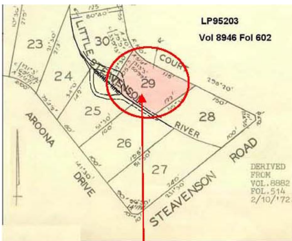
A re-establishment of lot 29 should maintain the position of Little Steavenson River as located in the parent survey.
