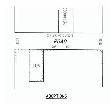
PS400000 has been assessed at an acceptable re-establishment of LP10000 and, consequently, is suitable to use as an initial datum for the survey of the LUS.
