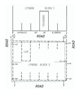
You have been asked to re-establish a lot within Block 2 of a large subdivision, LP10000. There are no registered surveys in the block; however, one exists in the block immediately to the north, namely PS400000.
